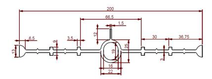
Centrally placed Waterbar, suitable for expansion joints. Installation in the centre of concrete structures. Easy anchoring of Sika Waterbar® O-20 SH to reinforcement with special fixing clips (5 pieces per m). Junction / Jointing Pieces: For welding waterbar pieces and cuts on site, special equipment is supplied.
